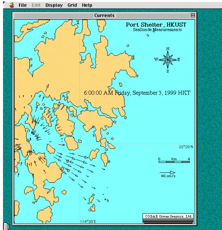
Fig. 2 Codar output indicating the ocean current
